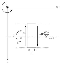
$$w|_{atx=0} = \frac{\partial w}{\partial x} \Big|_{atx=0} = 0, \quad \frac{\partial^2 w}{\partial x^2} \Big|_{atx=L} = 0$$
